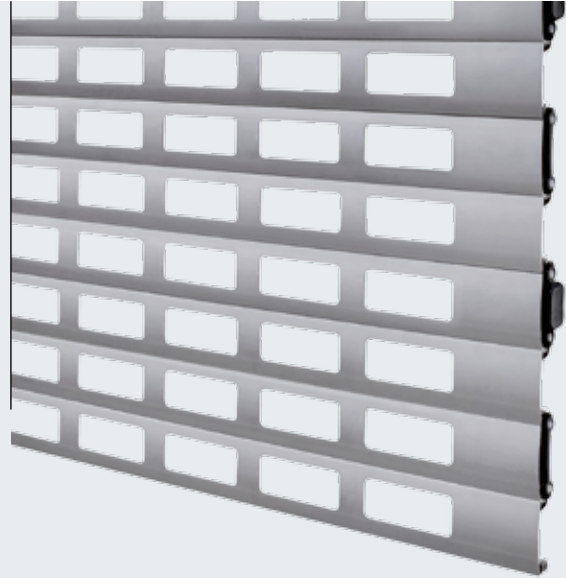
HG 75, aluminium The extruded aluminium profiles are available in a powder-coated surface finish. The 100 x 40 mm square holes can be provided in a straight or offset arrangement.
